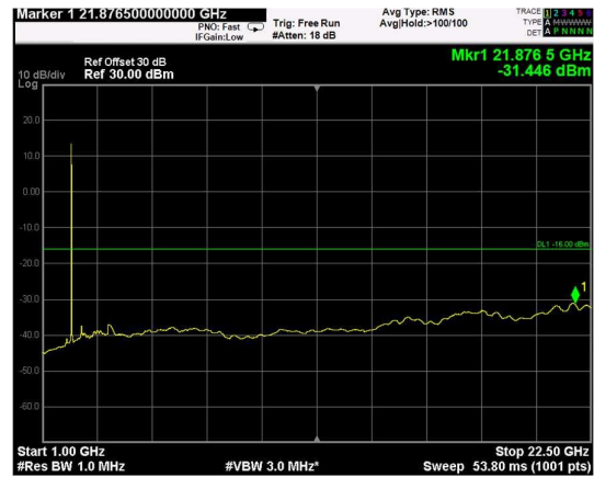
Channel: BOTTOM, Modulation: 256QAM, BW=5MHz, Range: Upper
