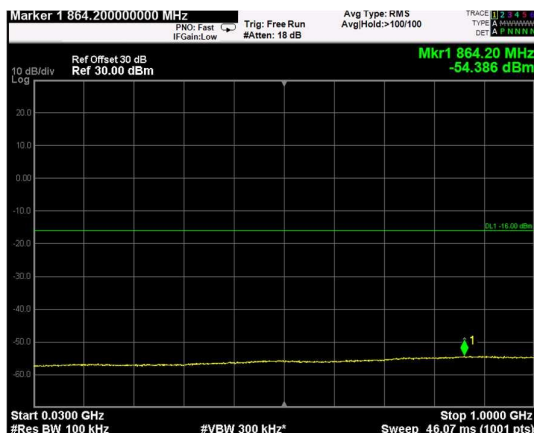
Channel: TOP, Modulation: 64QAM, BW=5MHz, Range: Lower
