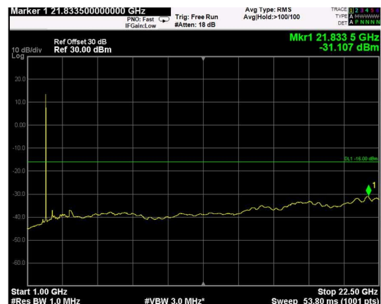
Channel: TOP, Modulation: 256QAM, BW=5MHz, Range: Upper
