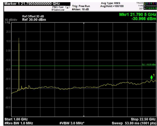
Channel: BOTTOM, Modulation: 16QAM, BW=10MHz, Range: Upper
