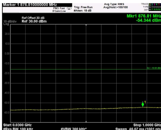
Channel: TOP, Modulation: 16QAM, BW=5MHz, Range: Lower
