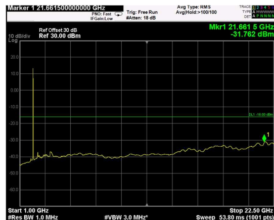
Channel: TOP, Modulation: 16QAM, BW=10MHz, Range: Upper
