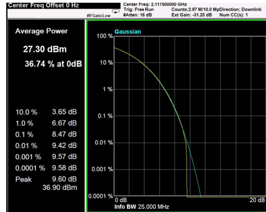
Channel: BOTTOM, Modulation: 256QAM, BW=15MHz, CCDF
