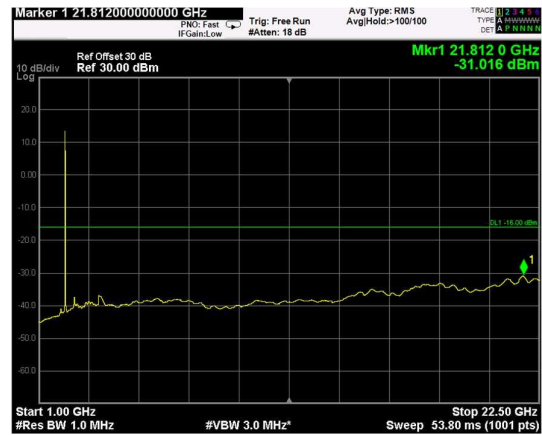
Channel: BOTTOM, Modulation: 64QAM, BW=10MHz, Range: Upper
