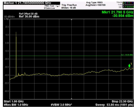
Channel: MIDDLE, Modulation: QPSK, BW=10MHz, Range: Upper
