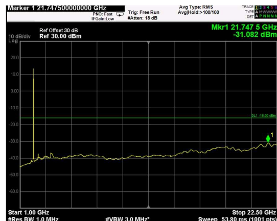
Channel: TOP, Modulation: 16QAM, BW=5MHz, Range: Upper
