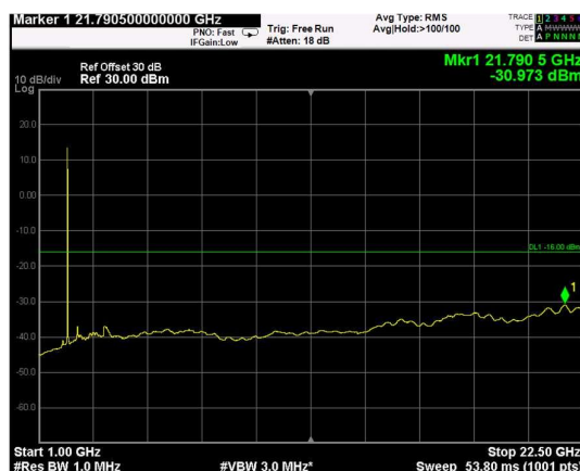
Channel: MIDDLE, Modulation: QPSK, BW=5MHz, Range: Upper
