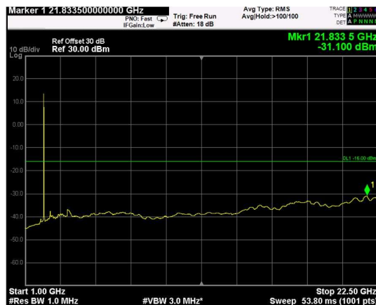
Channel: BOTTOM, Modulation: 64QAM, BW=5MHz, Range: Upper
