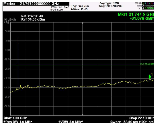
Channel: MIDDLE, Modulation: 64QAM, BW=5MHz, Range: Upper
