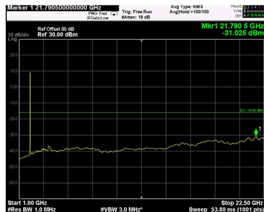
Channel: TOP, Modulation: 16QAM, BW=10MHz, Range: Upper
