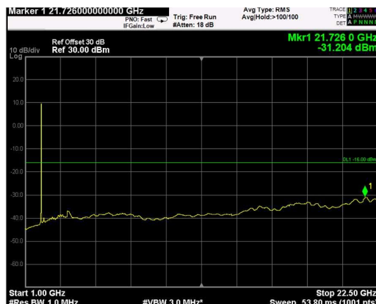
Channel: TOP, Modulation: 256QAM, BW=20MHz, Range: Upper
