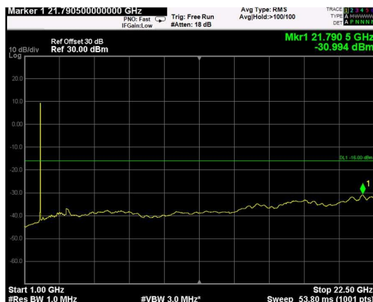
Channel: TOP, Modulation: 256QAM, BW=5MHz, Range: Upper
