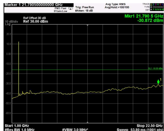
Channel: TOP, Modulation: 64QAM, BW=20MHz, Range: Upper
