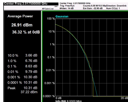
Channel: TOP, Modulation: 256QAM, BW=5MHz, CCDF
