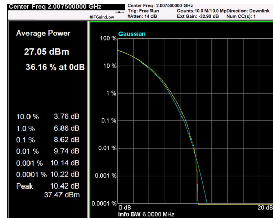
Channel: MIDDLE, Modulation: 256QAM, BW=5MHz, CCDF
