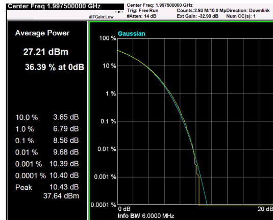
Channel: BOTTOM, Modulation: QPSK, BW=5MHz, CCDF
