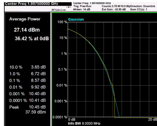
Channel: BOTTOM, Modulation: 64QAM, BW=5MHz, CCDF
