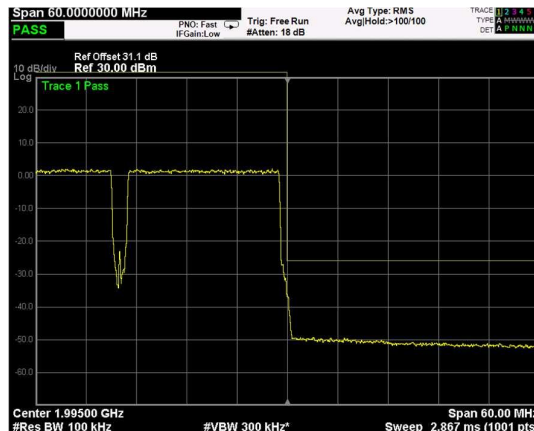
High Band Edge, 2 Carrier, Modulation: 16QAM, BW=20MHz
