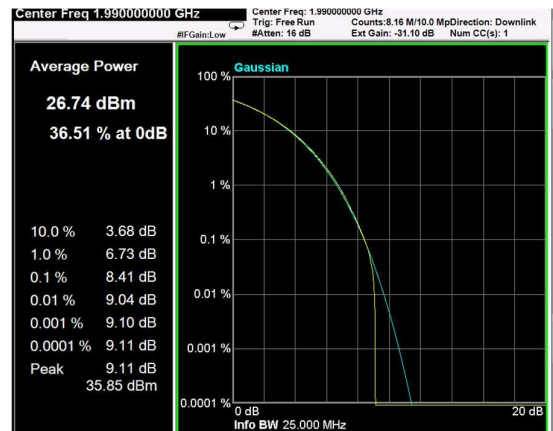
Channel: TOP, Modulation: 64QAM, BW=10MHz, CCDF
