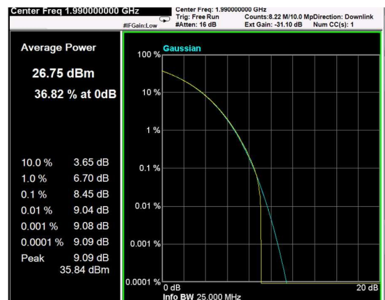
Channel: TOP, Modulation: 16QAM, BW=10MHz, CCDF
