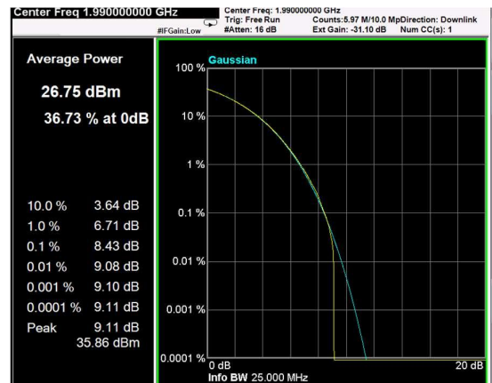
Channel: TOP, Modulation: 256QAM, BW=10MHz, CCDF
