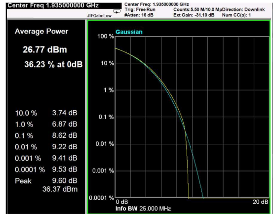
Channel: BOTTOM, Modulation: 256QAM, BW=10MHz, CCDF
