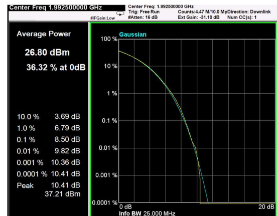
Channel: TOP, Modulation: QPSK, BW=5MHz, CCDF
