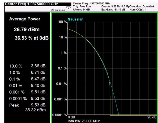
Channel: TOP, Modulation: 256QAM, BW=15MHz, CCDF
