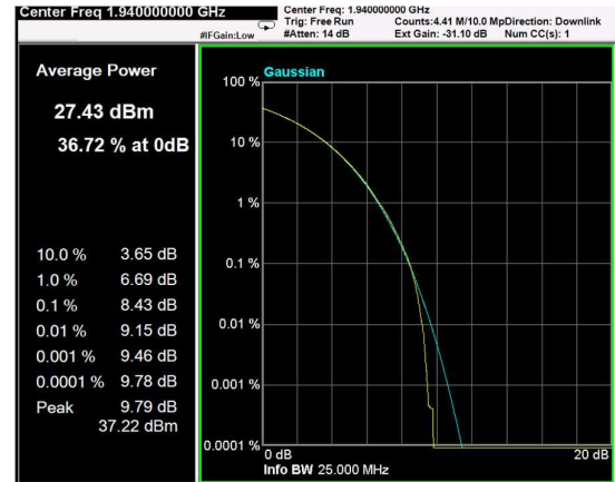
Channel: BOTTOM, Modulation: 64QAM, BW=20MHz, CCDF
