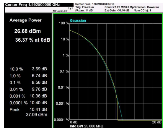
Channel: TOP, Modulation: 16QAM, BW=5MHz, CCDF
