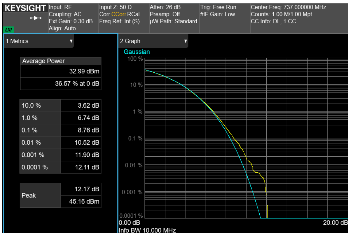
10 MHz signal, middle channel, nominal input signal
