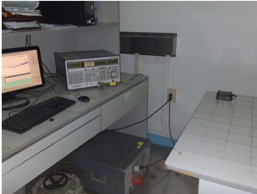
Photograph 2: Set-up for measurement of radiated emission, <1GHz
