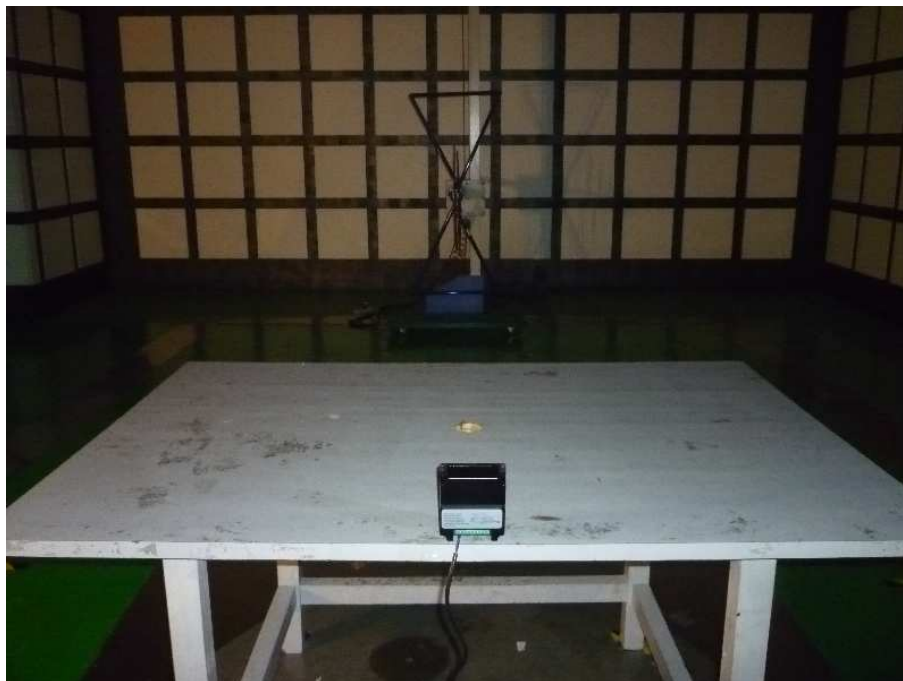
Photograph 2: Set-up for measurement of radiated emission, <1GHz
