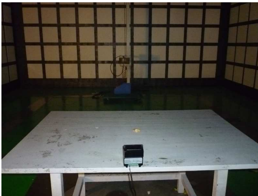
Photograph 3: Set-up for measurement of radiated emission, >1GHz
