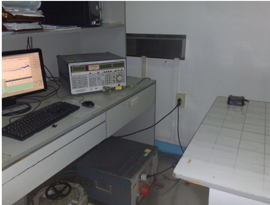
Photograph 2: Set-up for measurement of radiated emission, <math><1\text{GHz}</math>
