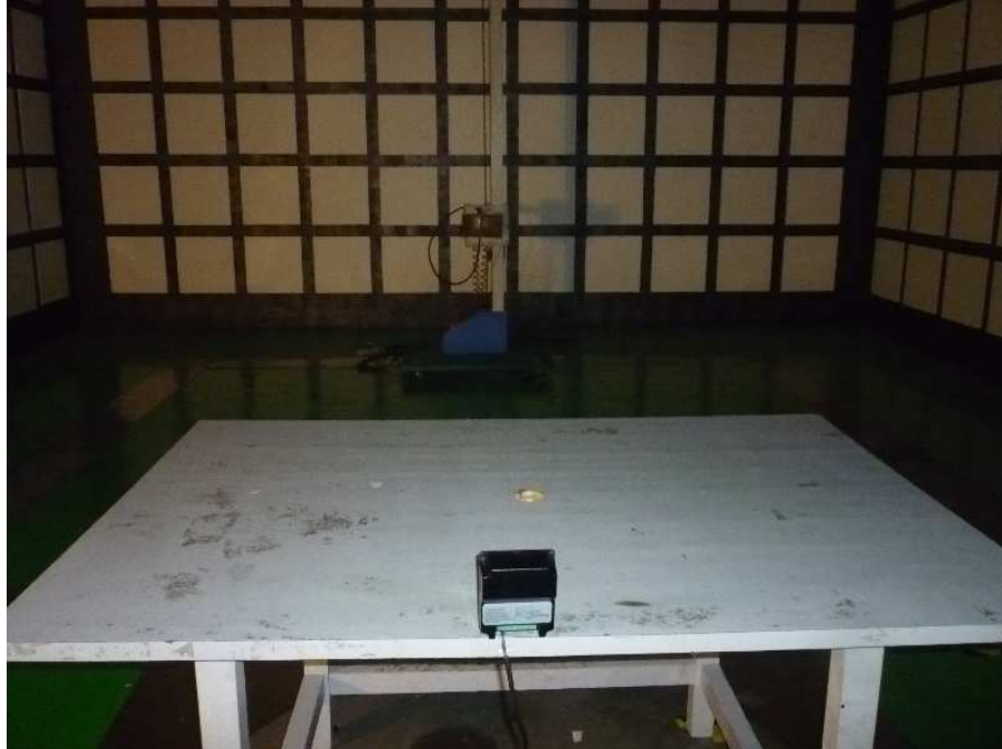
Photograph 3: Set-up for measurement of radiated emission, >1GHz
