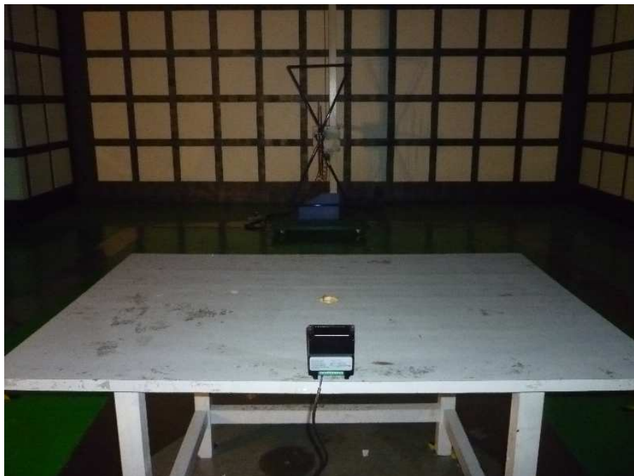
Photograph 2: Set-up for measurement of radiated emission, <math><1\text{GHz}</math>
