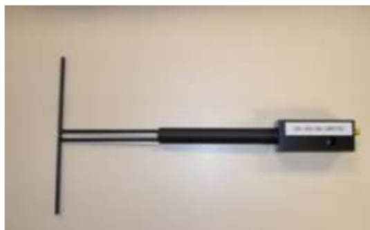
Figure 1 – Satimo COMOSAR Validation Dipole
