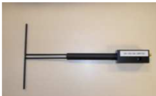
Figure 1 – Satimo COMOSAR Validation Dipole
