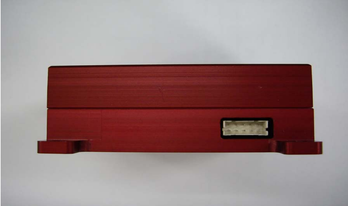
Figure 7 - FS-GM201 Reader Connections (GPIO Connector) |
