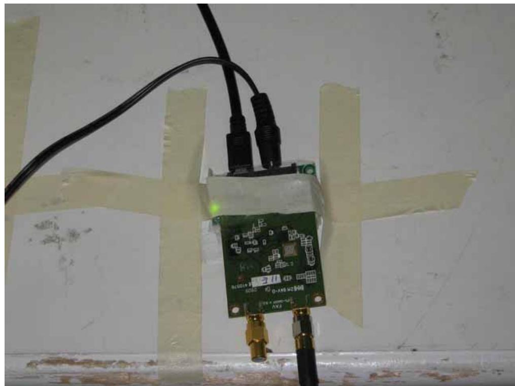
**RADIATED RF MEASUREMENT SETUP**
