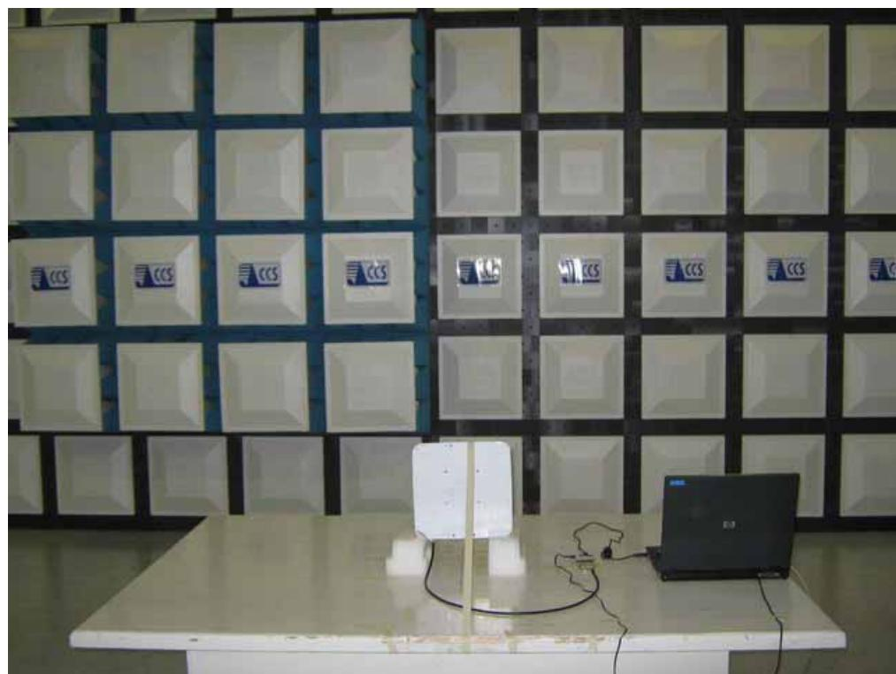
ANTENNA PORT CONDUCTED RF MEASUREMENT SETUP
