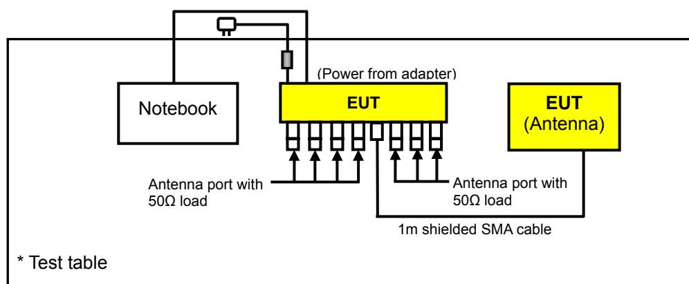
\* The EUT has 8 tx ports and supports tx diversity function, but only one port can transmit at a time.
