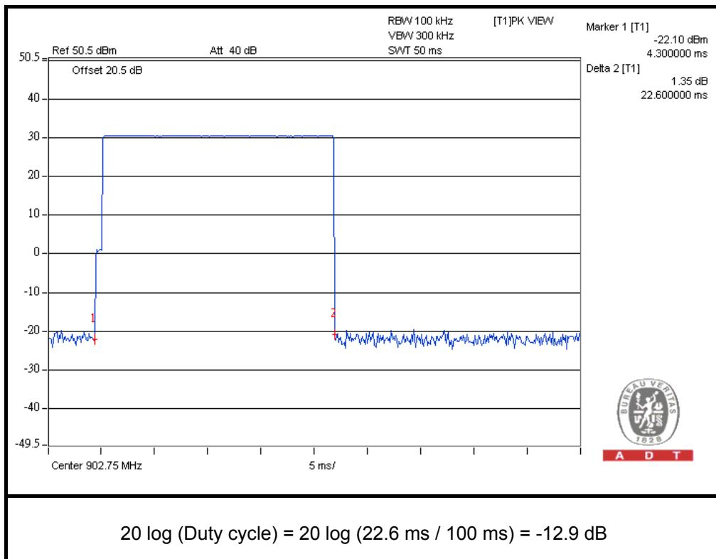
$$20 \log (\text{Duty cycle}) = 20 \log (22.6 \text{ ms} / 100 \text{ ms}) = -12.9 \text{ dB}$$
