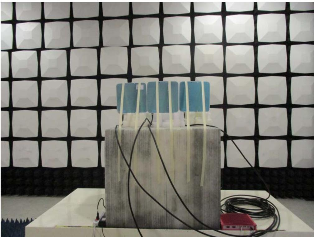
**ANTENNA PORT CONDUCTED RF MEASUREMENT SETUP**
