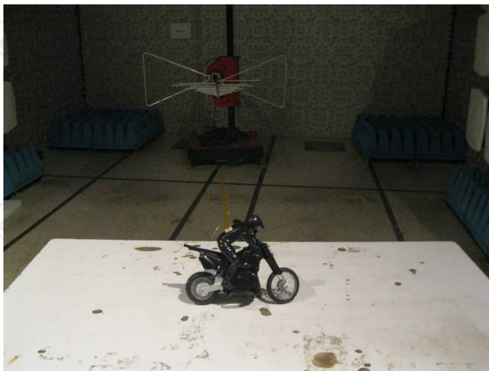
RADIATED EMISSION TEST SETUP (FOR RECEIVING MODE)
