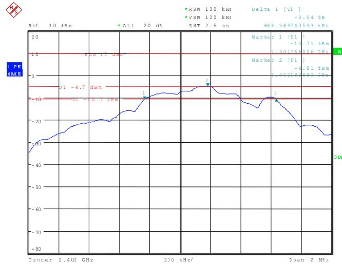
112920\_61.wmf: 6 dB bandwidth at the middle of the assigned frequency band:
