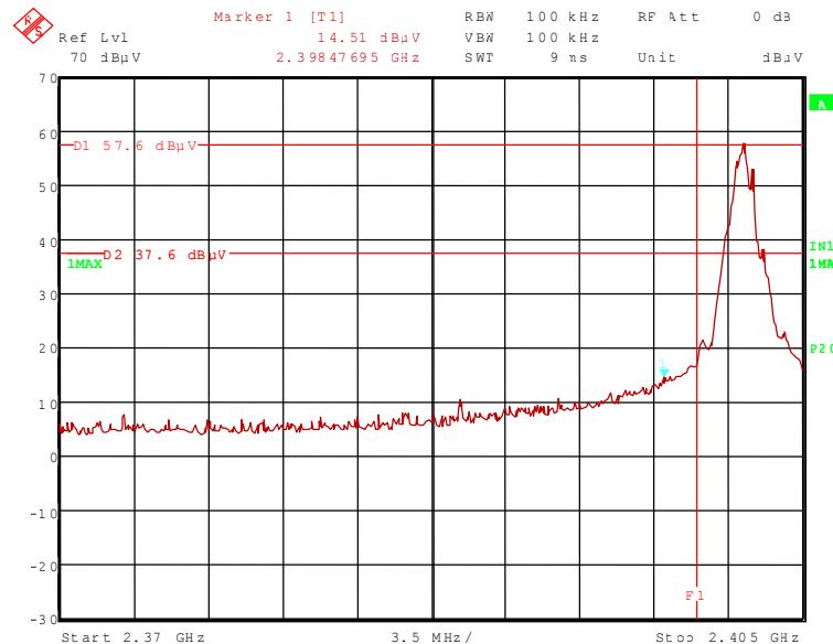
112920\_12.wmf: Radiated band-edge compliance, upper band edge (operation mode 3):
