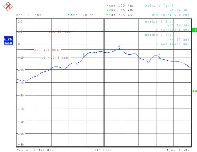
112920\_62.wmf: 6 dB bandwidth at the upper end of the assigned frequency band:
