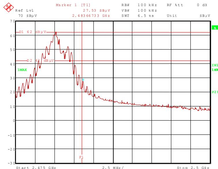
The plots on the page before are showing the radiated band-edge compliance for the upper band-edge. The display line 1 (D1) in these plots represents the highest level within the assigned frequency band. The display line 2 (D2) represents the 20 dB offset to this highest level and shows the compliance with FCC 47 CFR Part 15.247 (d). The frequency line 1 (F1) shows the edge of the assigned frequency.
