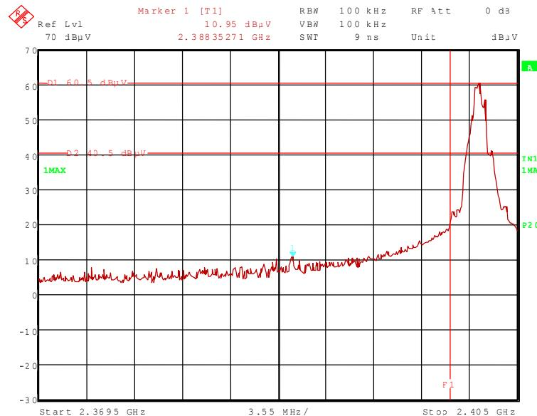
112920\_2.wmf: Radiated band-edge compliance, upper band edge (operation mode 3):
