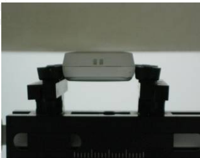
Fig.3 Testing body-worn SAR the front side of the EUT is paralleled and contact with flat phantom in GPRS mode.
