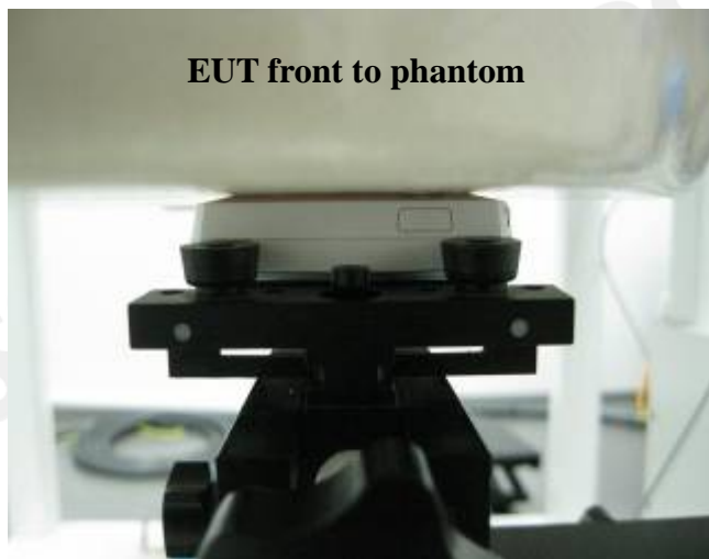
Fig.3 Testing body-worn SAR the front side of the EUT is paralleled and contact with flat phantom in GPRS mode.
