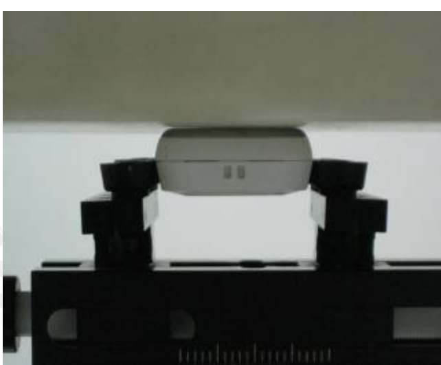
Fig.4 Testing body-worn SAR the back side of the EUT is paralleled and contact with flat phantom in GPRS mode.
