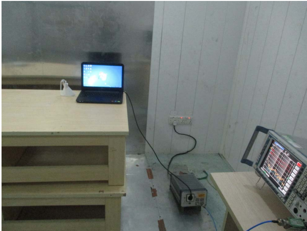
FCC RADIATED EMISSION TEST SETUP
