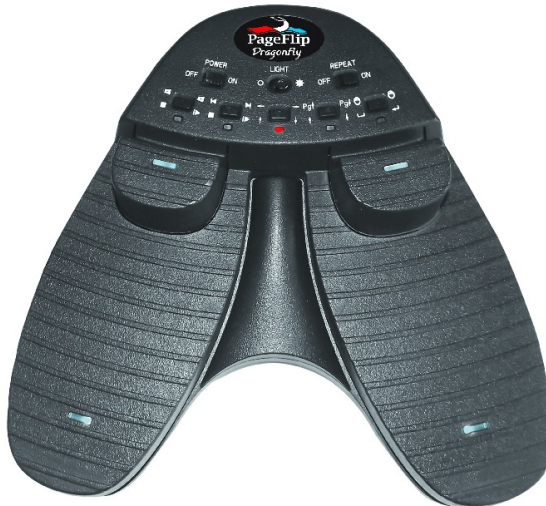
Figure 6: Primary (larger) and secondary (smaller) pedals. Each of these four pedals has an LED light that can be turned on for use in dim venues.
