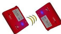
3. The acquisition of the readings is confirmed by the emission of a beep signal and by a brief lighting of the LED indicator. The number of readings got, shown on the display of the **RFIDat**, configured in the "Master" mode, is consequently increased.
