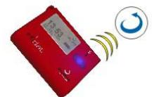
3. The TAG reading completion is confirmed by a short beep with the blue LED "on" for three seconds. Consequently, the number of readings performed, shown on the display, is increased by 1.
