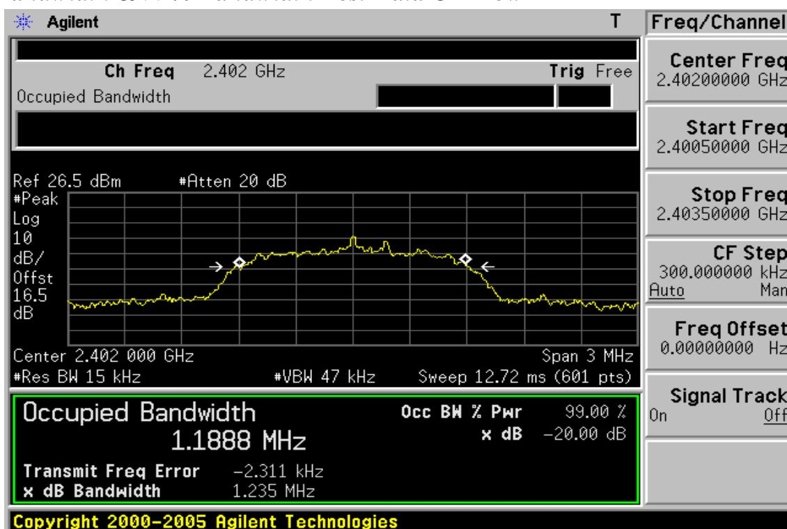
**20dB Bandwidth & 99% Bandwidth Test Data CH-Mid**
