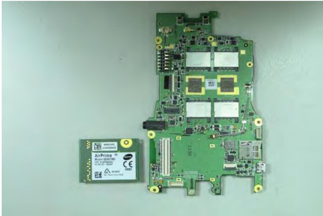
*Internal View of EUT - 8(2G module)*
