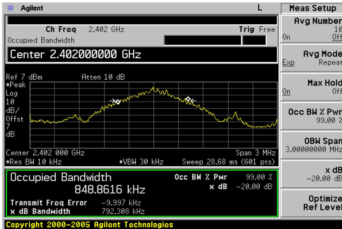
**20dB Bandwidth Test Data CH-Mid**
