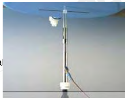
Photograph of the dipole Antenna
