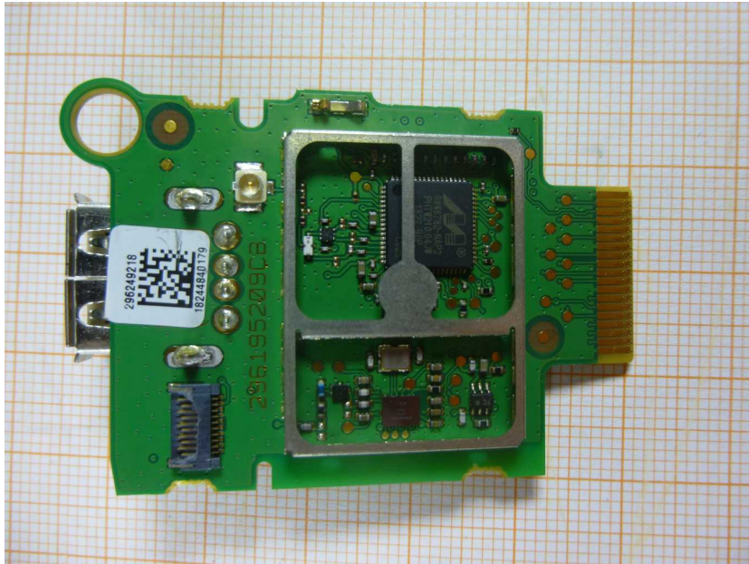
Photo 11: RF PCB front side view, shielding removed
