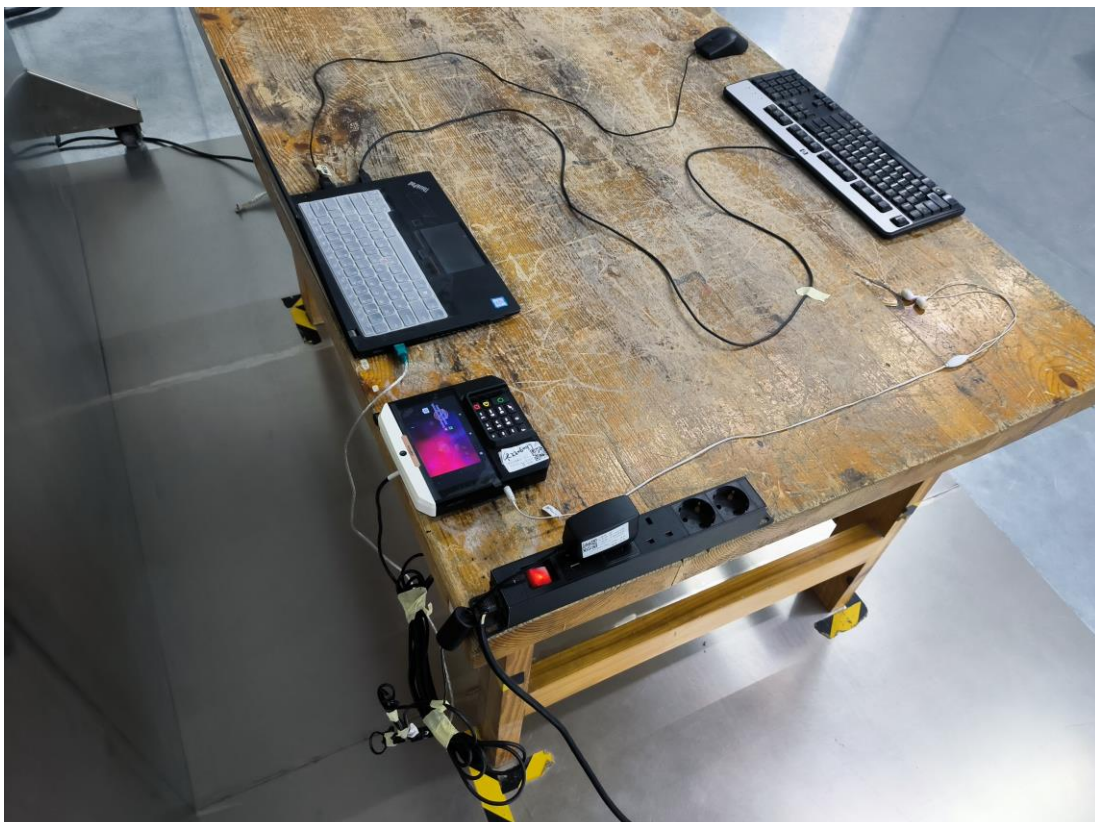
Conducted Emissions Side View M2
