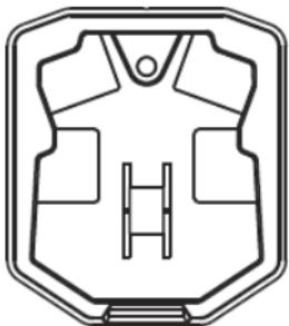
To fit the AXIUM RX5000 to the standpole, it only requires to slide down the AXIUM RX5000 until a click sound:
