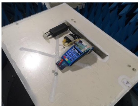
Test setup in anechoic chamber (9kHz to 1GHz)
