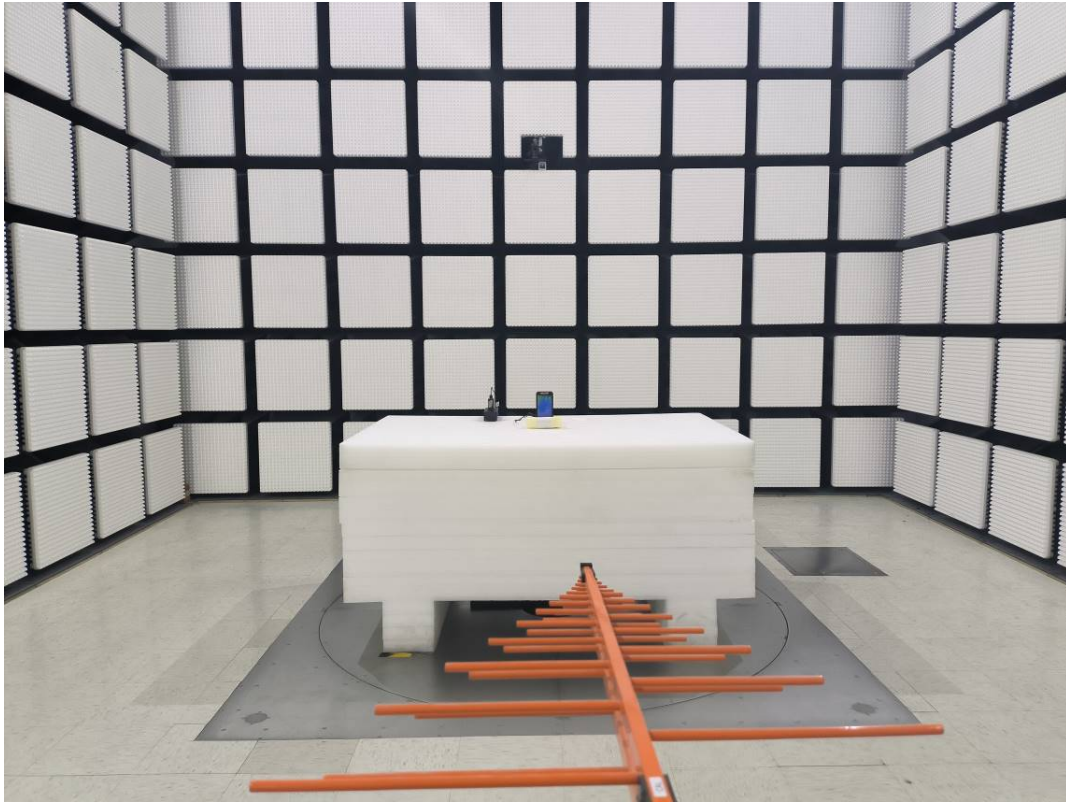
Radiated Emission Below 1GHz View-Adapter 4#+Configuration 1#
