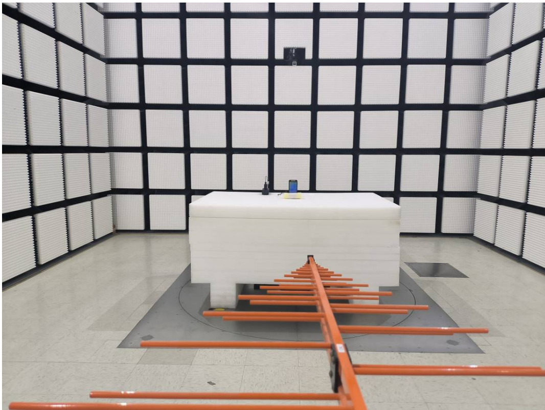
Radiated Emission Below 1GHz View-Adapter 4#+Configuration 1#
