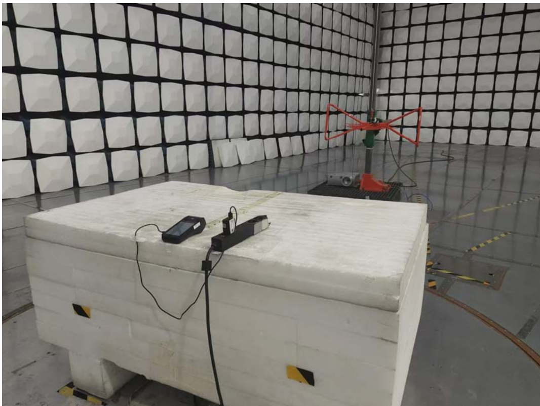
Radiated Emissions Below 1G side View M1-M5
