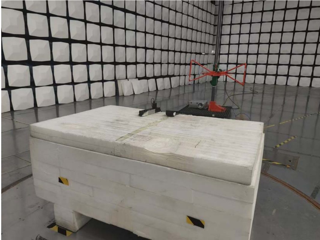
Radiated Emissions Below 1G side View M1-M5
