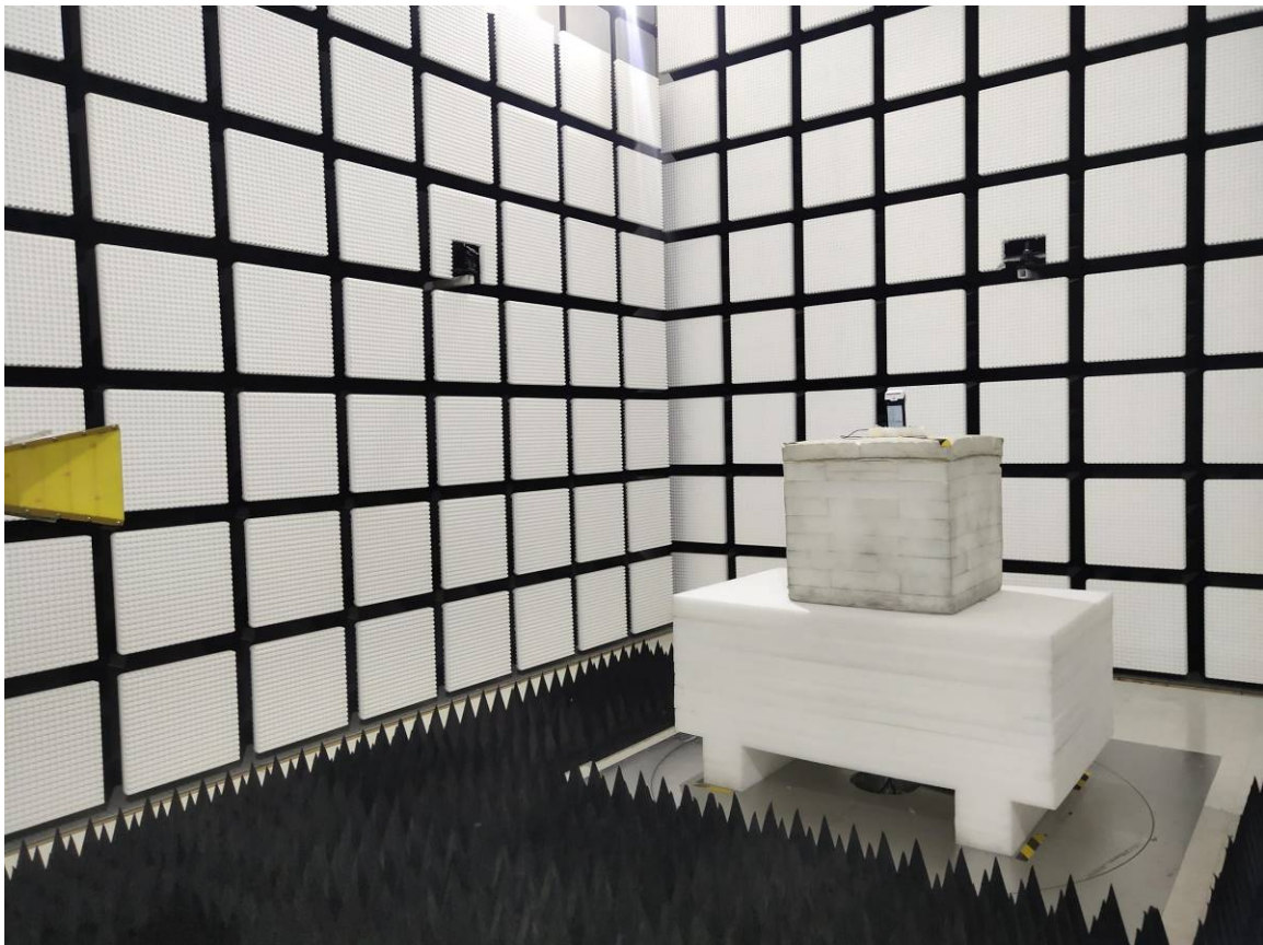
Radiated Emission Above 1GHz View-Adapter 4#
