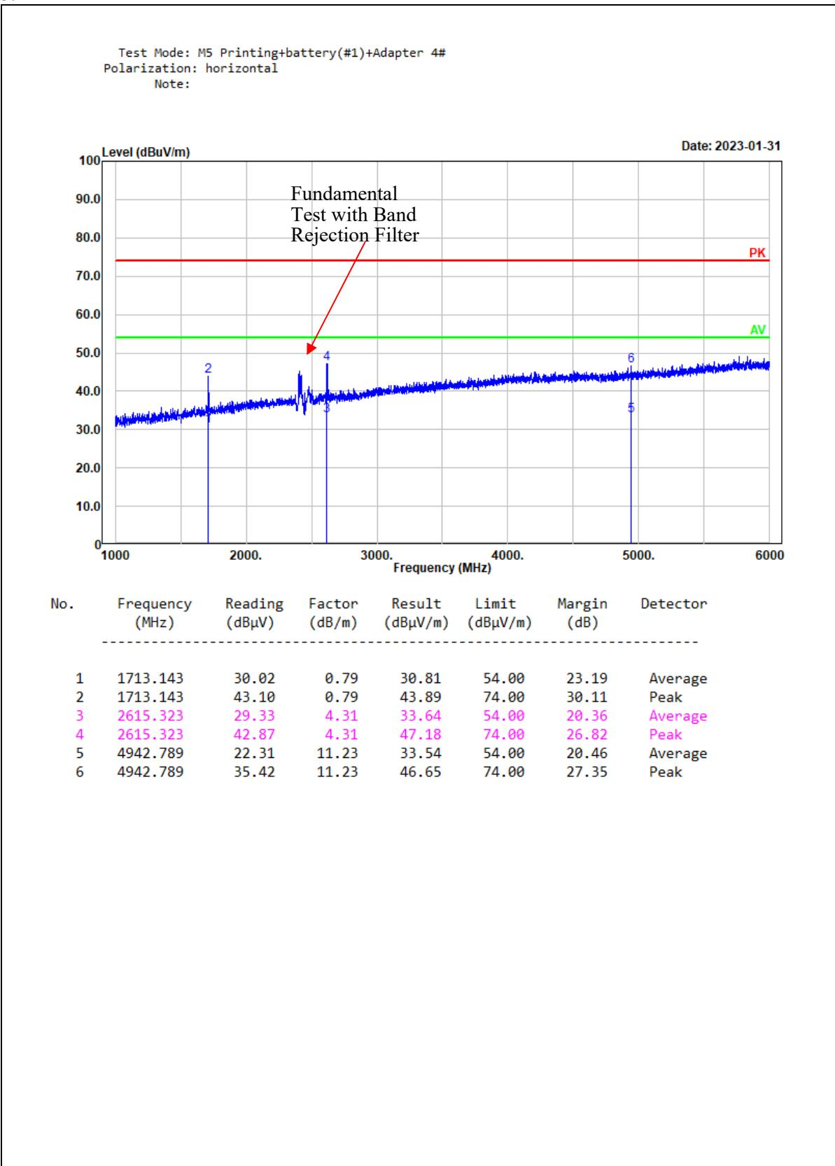
Test Mode: M5 Printing+battery(#1)+Adapter 4#
