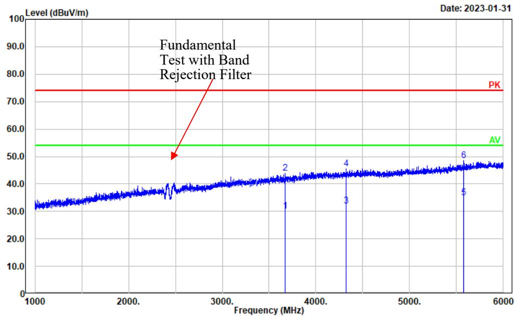
Test Mode: M4 Printing+battery(#1)+Adapter 3#
