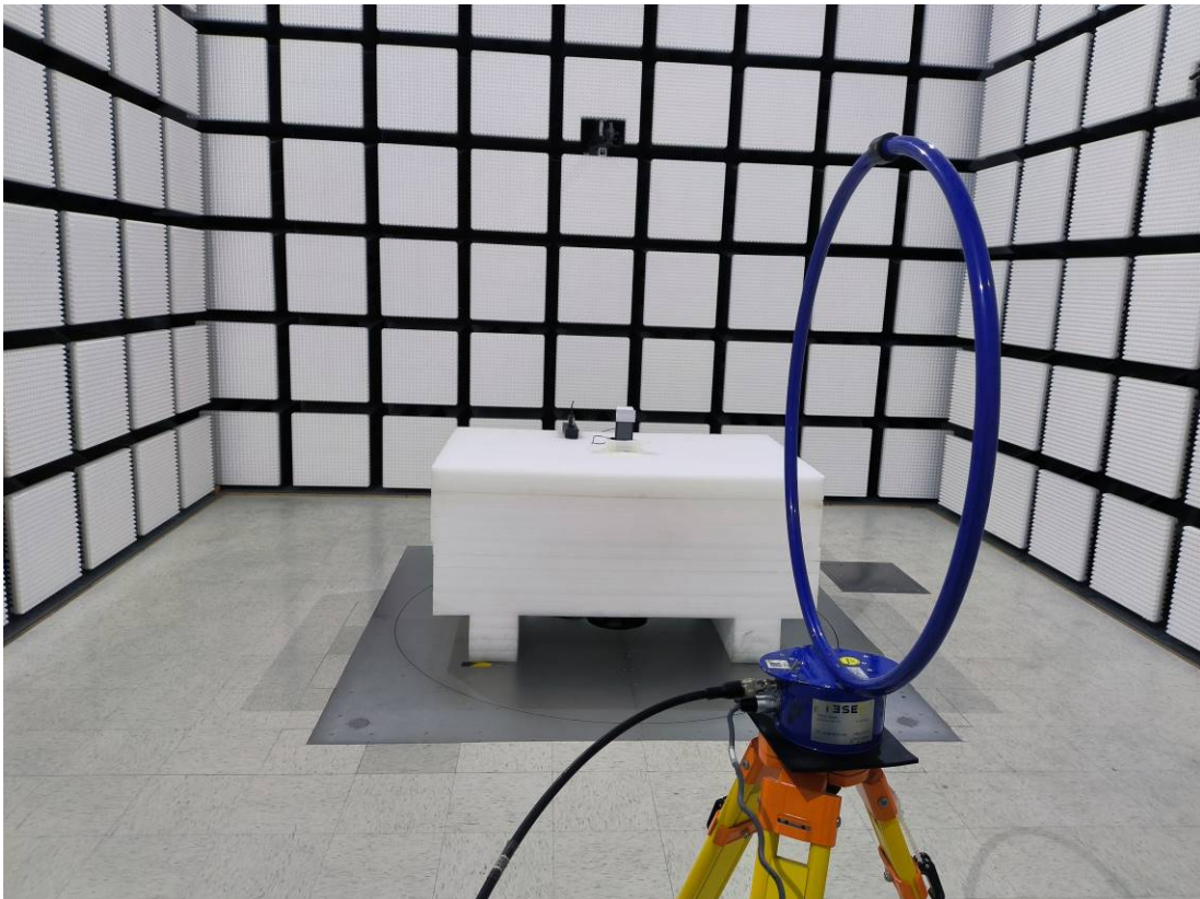
Radiated Emission 9k-30MHz Perpendicular View Adapter 4#
