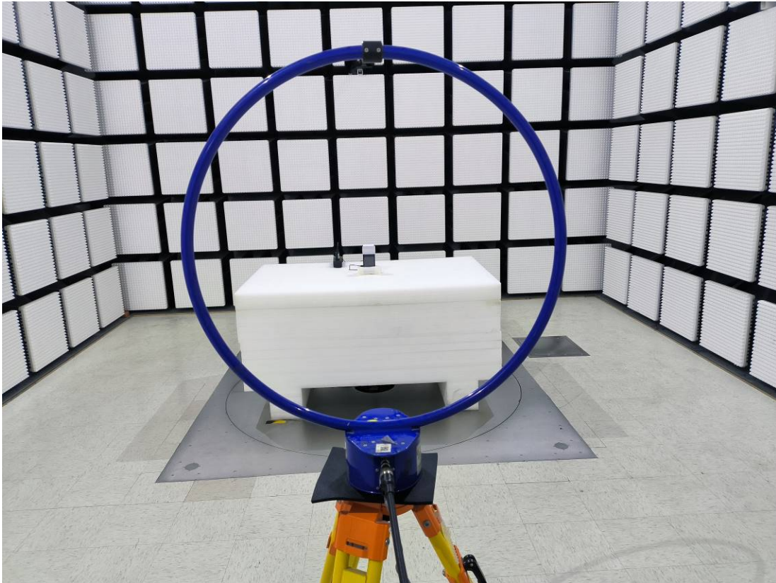
Radiated Emission 9k-30MHz Perpendicular View Adapter 4#
