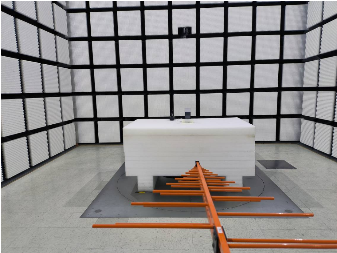
Radiated Emission 30M-1GHz View Adapter 4#
