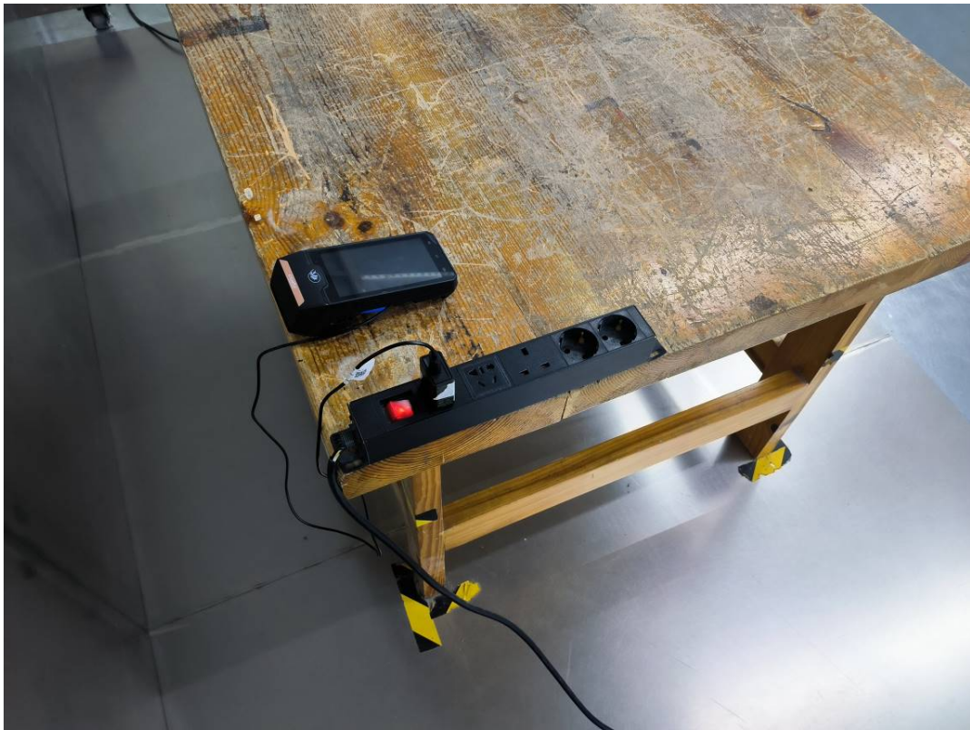
Conducted Emissions Side View Adapter 3# + TN
