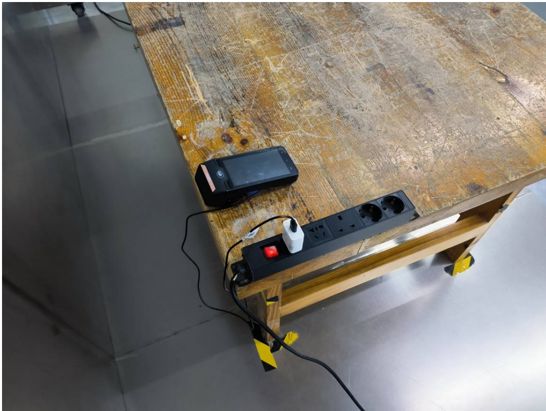
Conducted Emissions Side View Adapter 2# + TN
