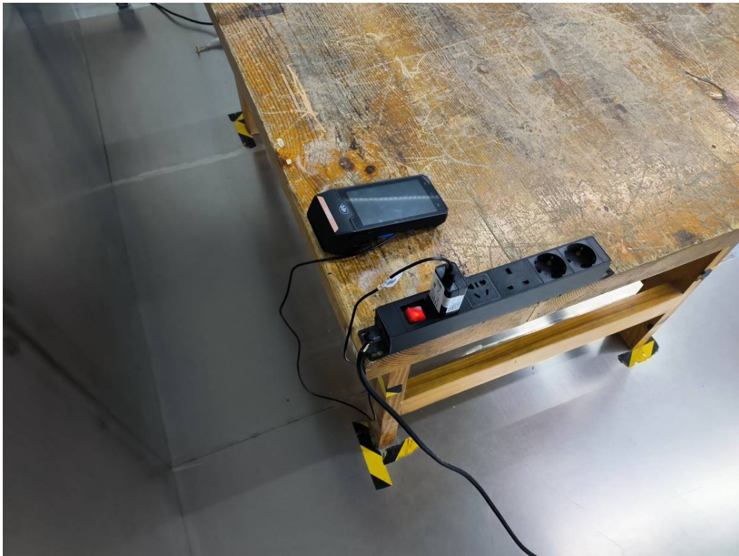
Conducted Emissions Side View Adapter 1# + TN
