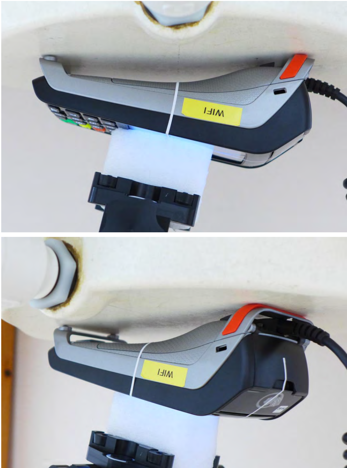
Pic. 5: Test position – back side, 0mm distance to phantom.
