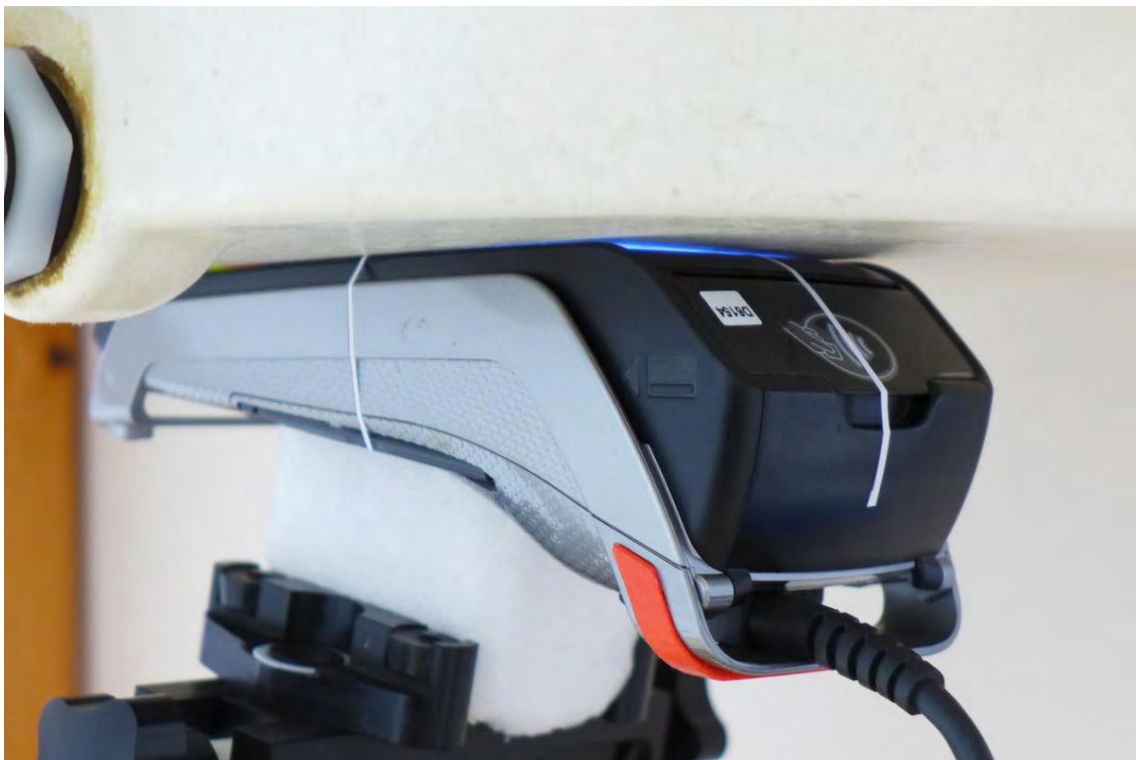
Pic. 3: Test position – front side, 0mm distance to phantom.
