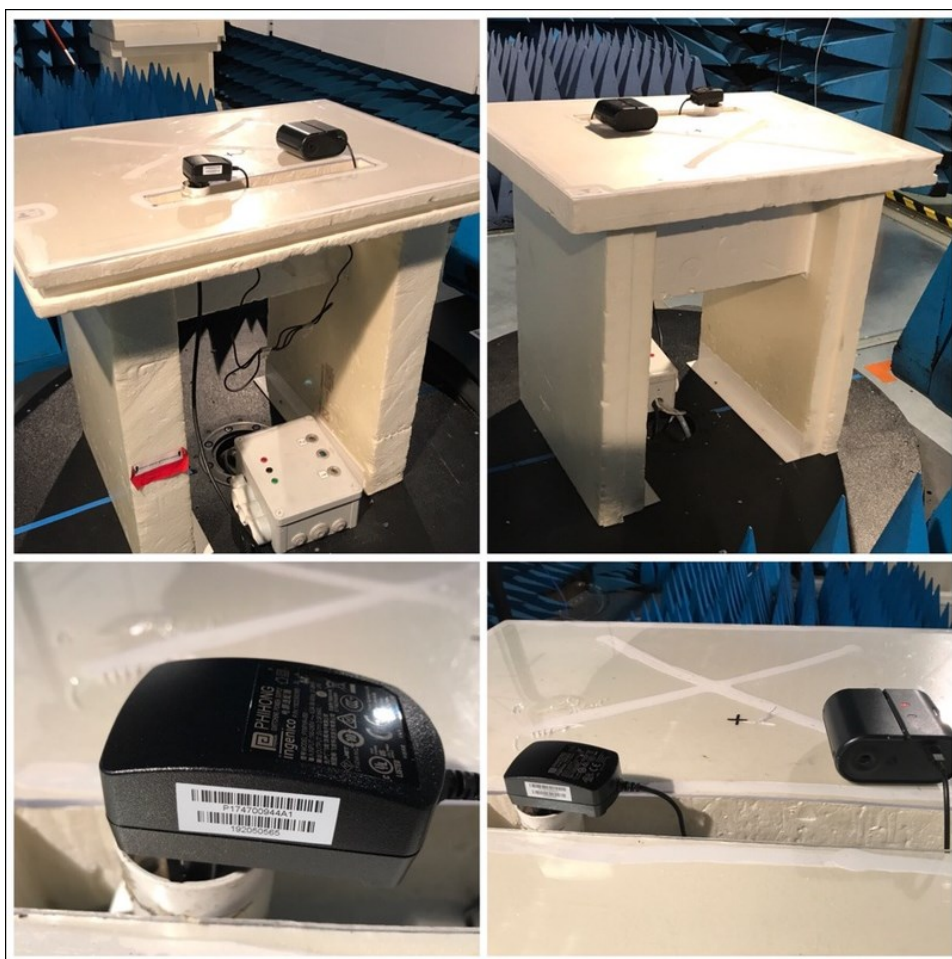
Test setup in anechoic chamber – Charging mode Cfg1 (<1Ghz) – EMC test setup
