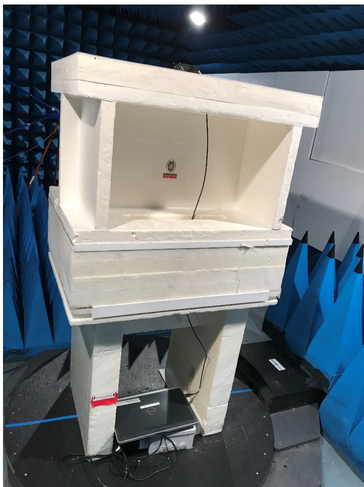
Test setup in anechoic chamber – Test setup (>1Ghz) -Configuration 4 DTM Test Mode
