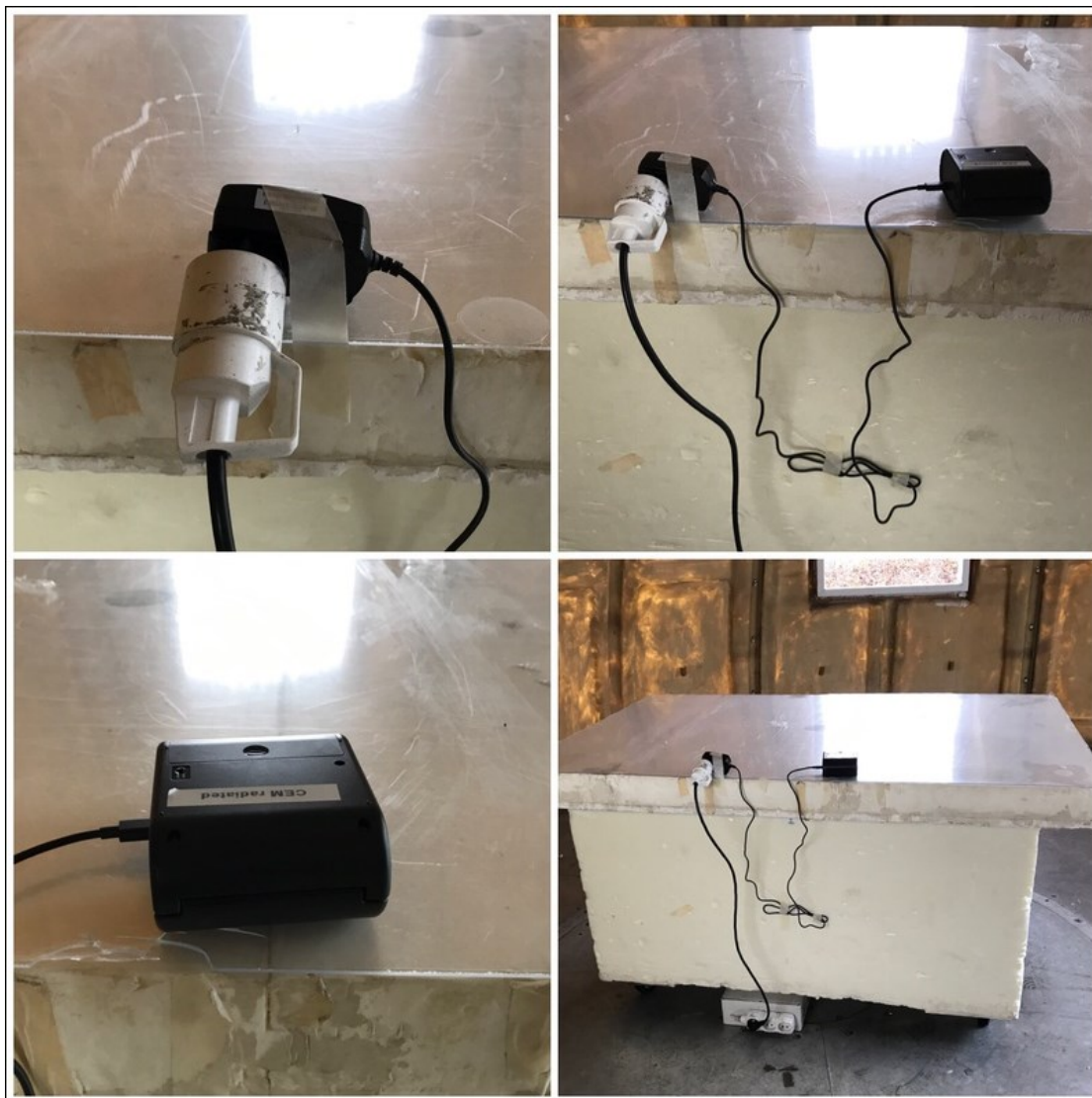
Test setup in OATS – Charging mode Cfg1 (<1Ghz) – EMC test setup
