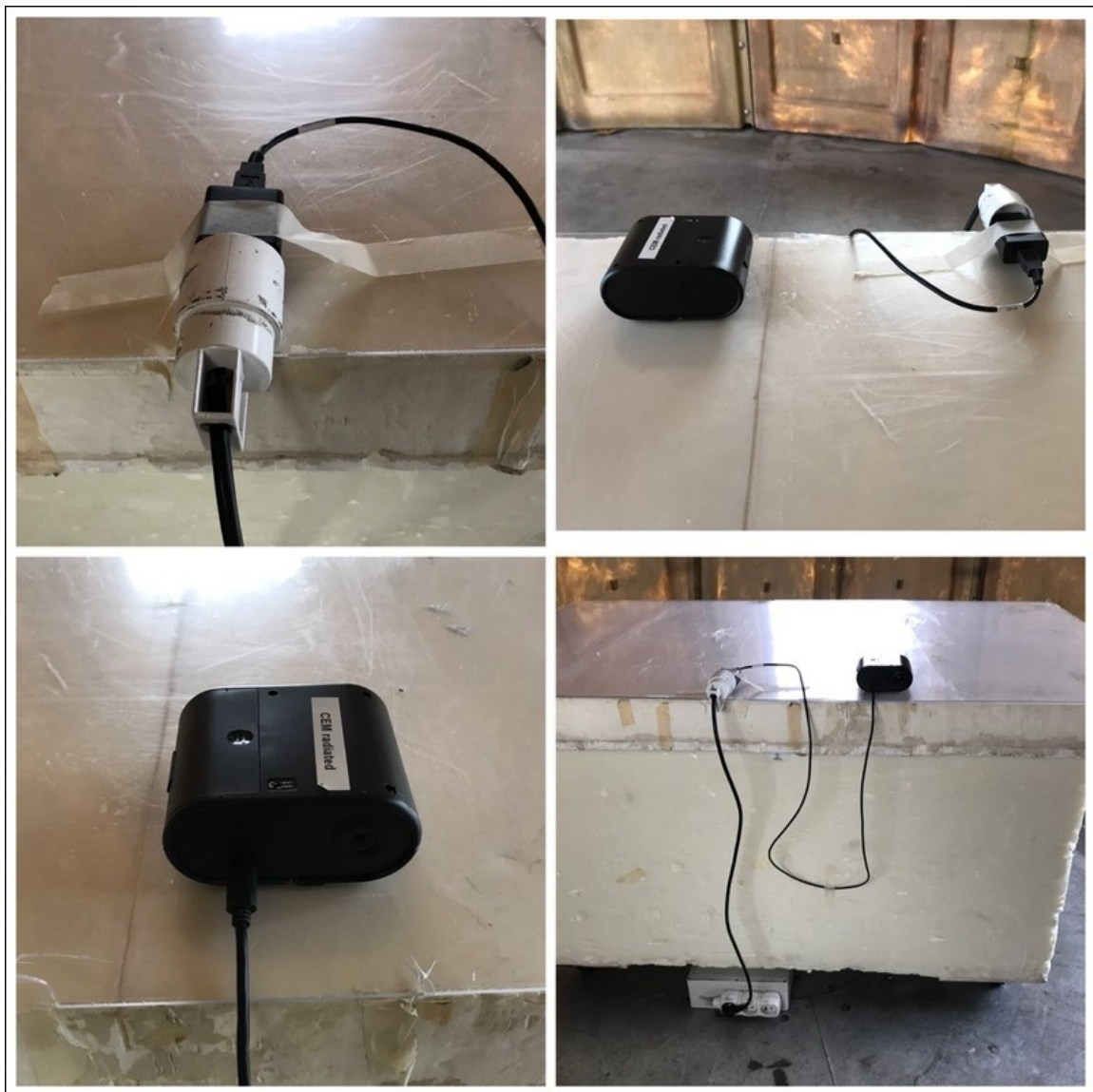
Test setup in OATS – Charging mode Cfg2(<1GHz) – EMC test setup
