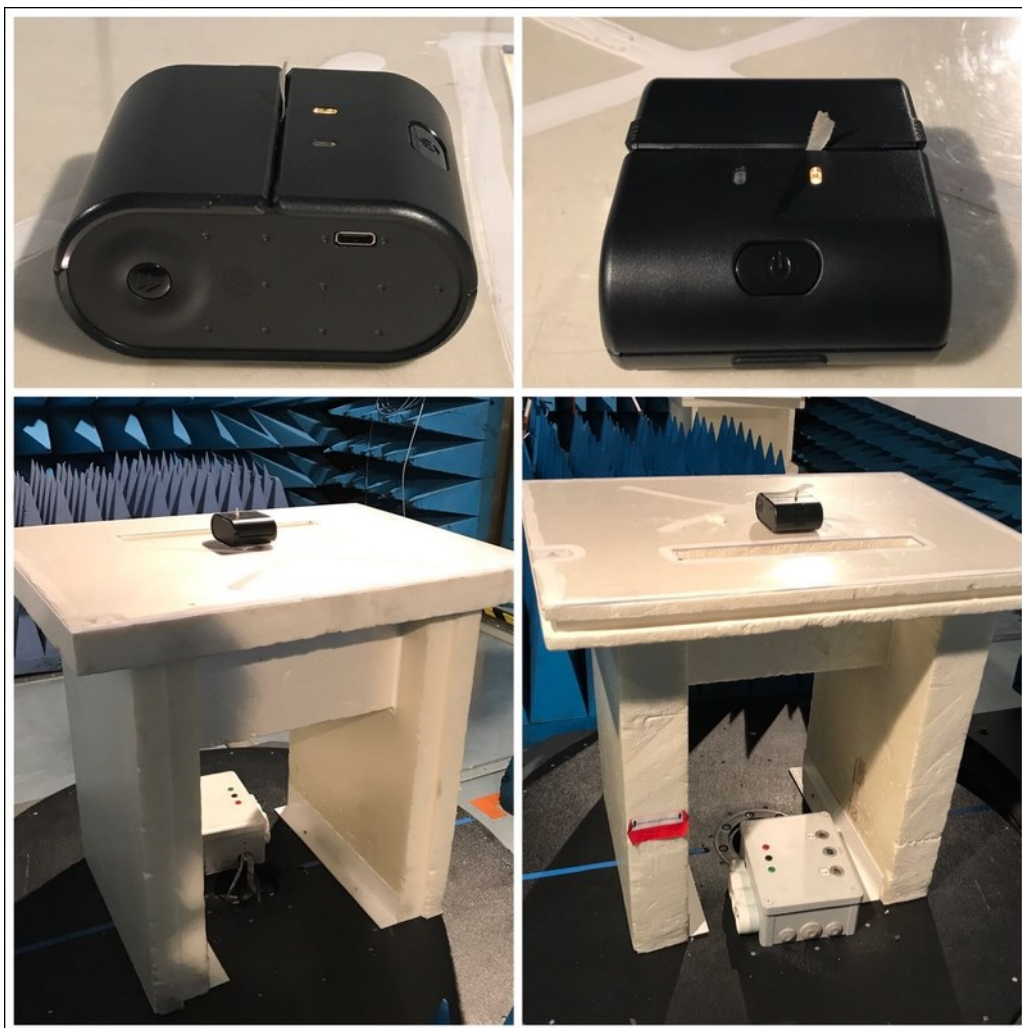
Test setup in anechoic chamber – Battery mode Cfg3(<1GHz) – EMC test setup
