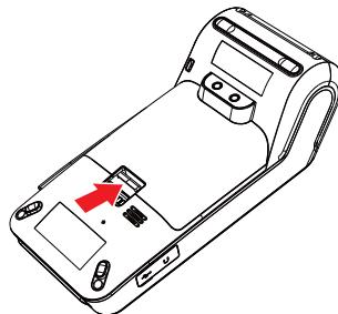
➤ Turn the terminal and remove the trapdoor.
