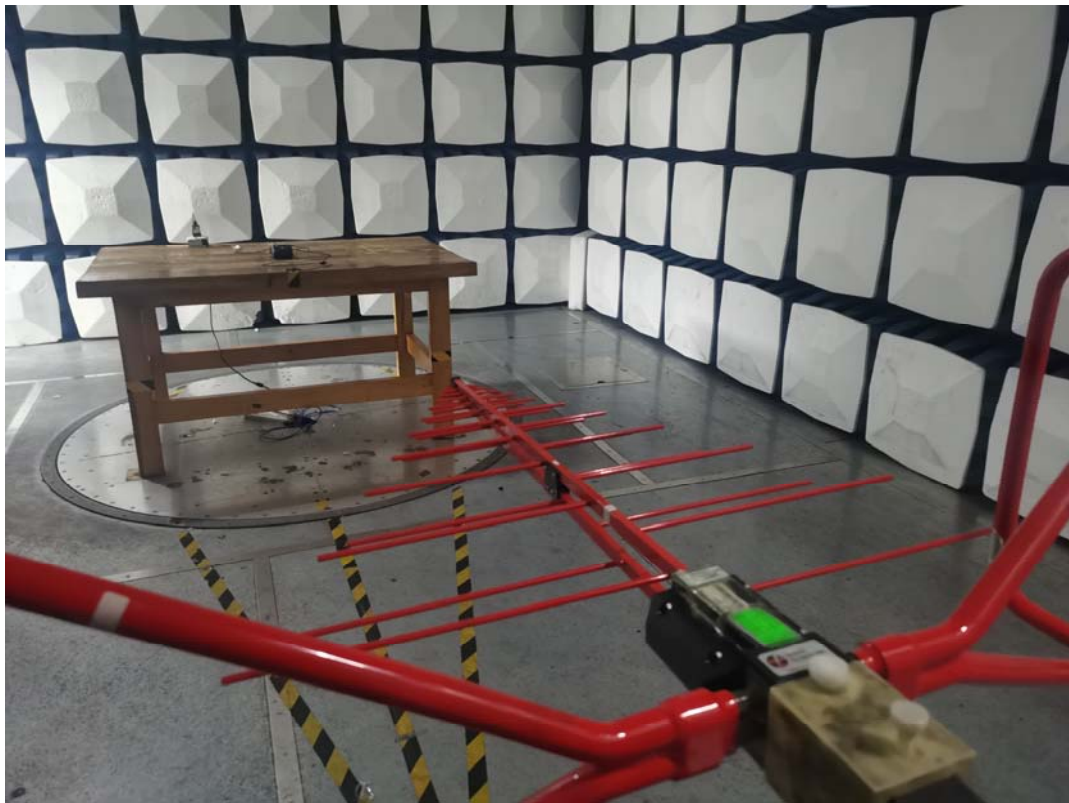
Radiated Emission Above 30MHz View
