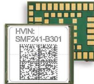
**HVIN: SMF241-B302** (RF Module with integrated metal sheet antenna)
