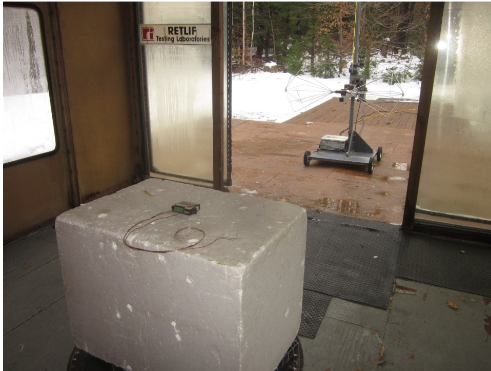
Horizontal Antenna Polarization, 30 MHz to 200 MHz, Biconical Antenna, Internal Antenna
