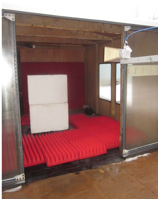
Vertical Antenna Polarization, 1 GHz to 18 GHz, Log Periodic, External Antenna
