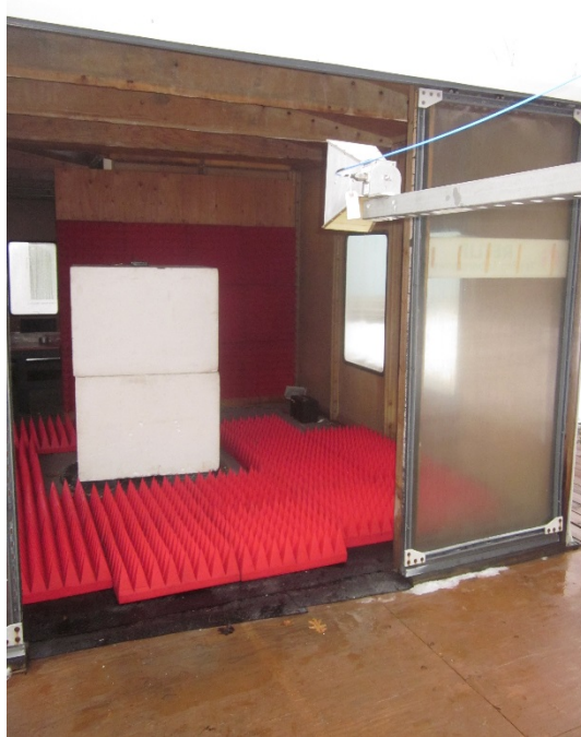
Horizontal Antenna Polarization, 1 MHz to 18 GHz, Log Periodic, Internal Antenna
