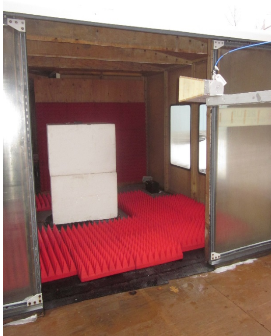
Vertical Antenna Polarization, 1 GHz to 18 GHz, Log Periodic, Internal Antenna
