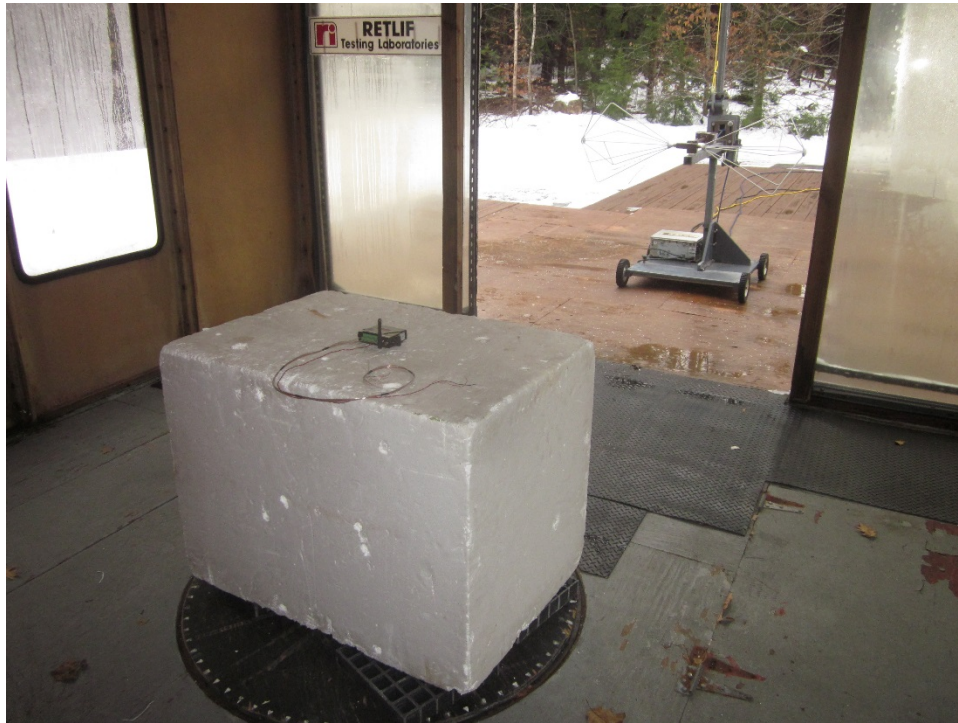
Horizontal Antenna Polarization, 30 MHz to 200 MHz, Biconical Antenna, External Antenna
