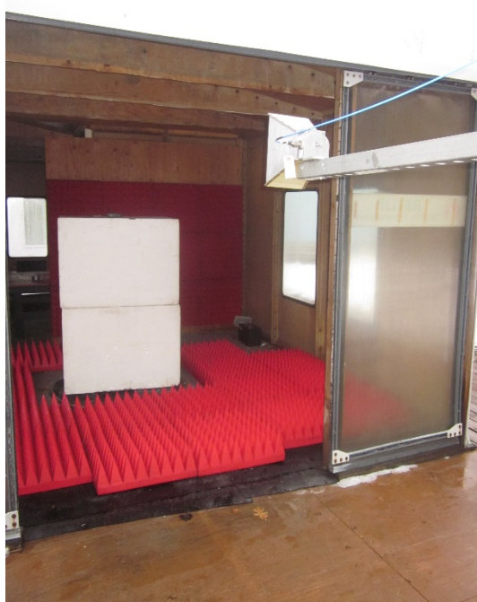
Horizontal Antenna Polarization, 1 GHz to 18 GHz, Log Periodic, External Antenna
