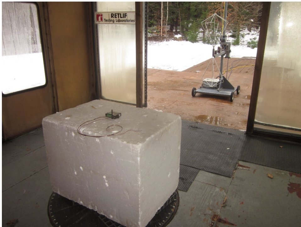
Vertical Antenna Polarization, 30 MHz to 200 MHz, Biconical Antenna, External Antenna
