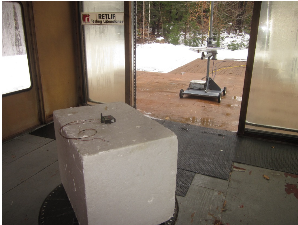
Horizontal Antenna Polarization, 200 MHz to 1 GHz, Log Periodic, External Antenna
