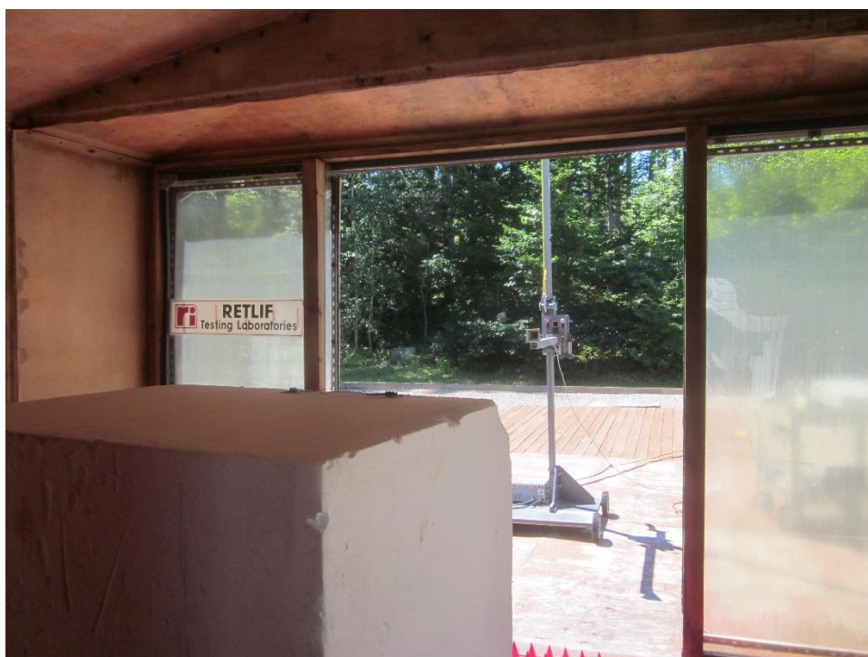
Vertical Antenna Polarization, 18 GHz to 25 GHz, Log Periodic Internal Antenna
