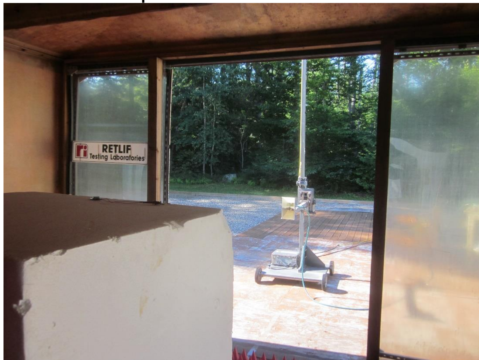
Horizontal Antenna Polarization, 1 MHz to 18 GHz, Log Periodic Internal Antenna
