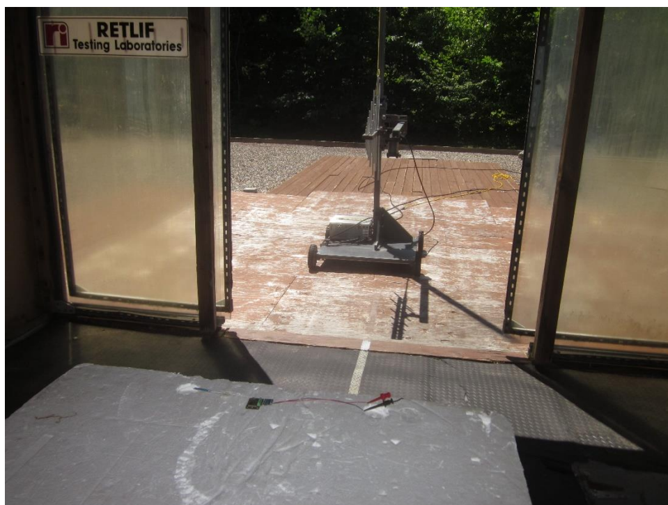
Vertical Antenna Polarization, 200 MHz to 1 GHz, Log Periodic, External Antenna
