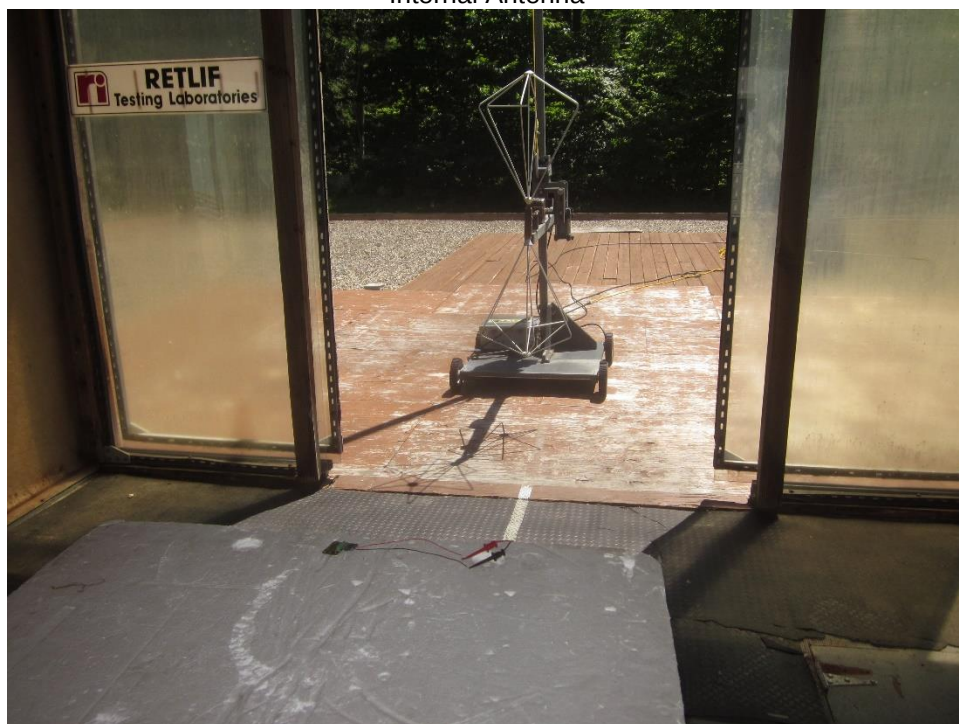
Vertical Antenna Polarization, 30 MHz to 200 MHz, Biconical Antenna Internal Antenna
