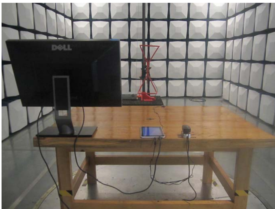
Radiated Emission - Rear View (Below 1GHz)
