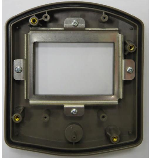
A photograph of the WPS LCD frame and front cover assembly. The frame is a dark, metallic-looking plastic housing that holds a white LCD screen. The screen is positioned in the center of the frame, which is secured with four screws. The frame has a rectangular shape with rounded corners.                                                                               |
