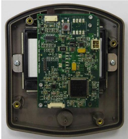
A photograph of the WPS front cover assembly, showing the internal circuit board. The board is green and densely populated with components, including a central microcontroller, various capacitors, and connectors. The text "HONEYWELL SENSING AND CONTROL" is visible on the board. The assembly is held in a clear plastic frame.                                           |
