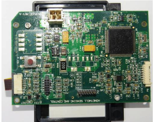
A photograph of the WPS LCD and Interface assembly. It shows a green printed circuit board (PCB) with various electronic components, including a central microcontroller, capacitors, and connectors. A black LCD screen is attached to the bottom of the PCB. The text "HONEYWELL SENSING AND CONTROL" is visible on the PCB. The assembly is held in a clear plastic frame. |
