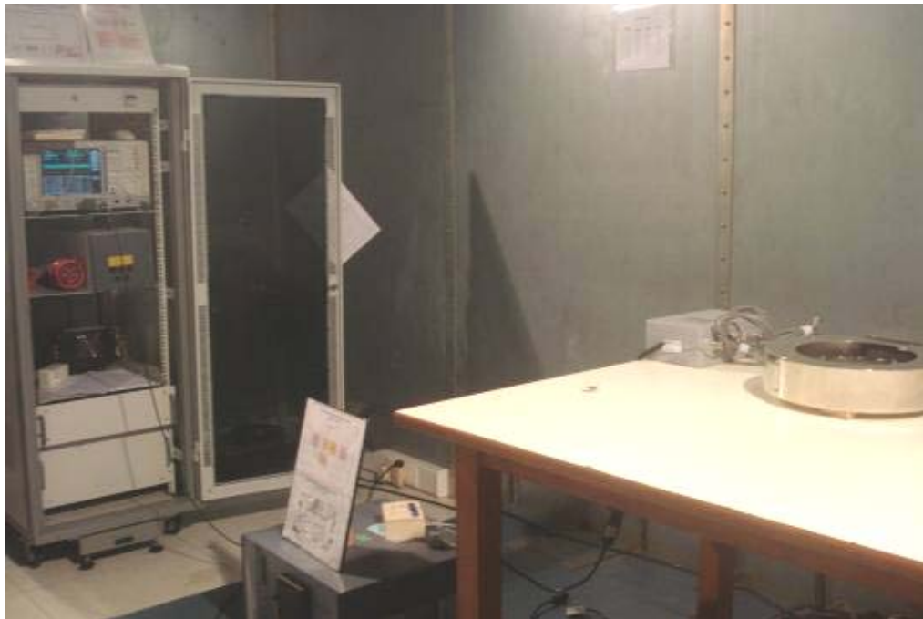
Conducted Emission Test Setup
