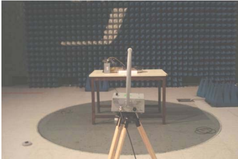
Radiated Emission Test Setup (Loop Antenna)
