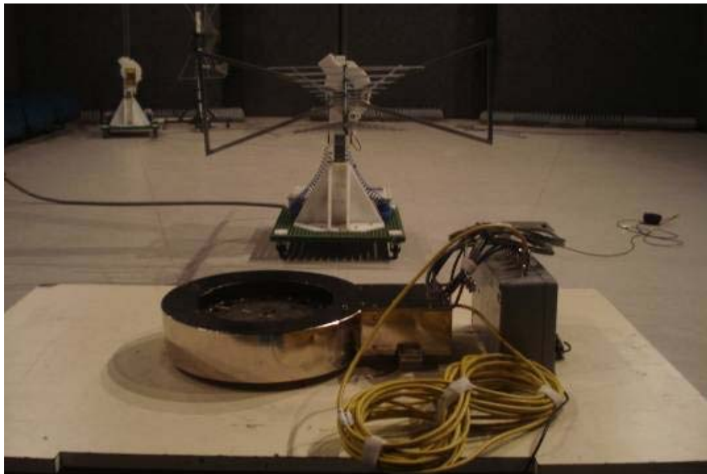
Radiated Emission Test Setup (Ultra Log Antenna)
