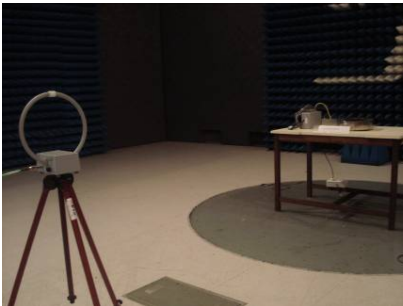
Radiated Emission Test Setup (Perpendicular)
