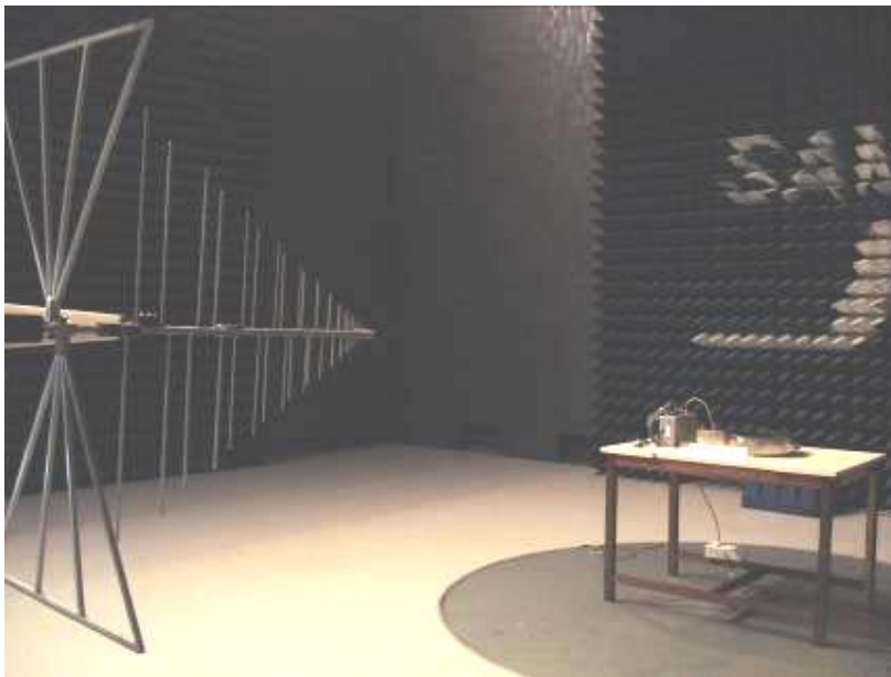
Radiated Emission Test Setup
