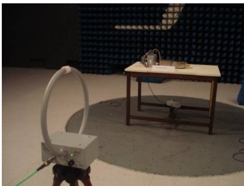
Radiated Emission Test Setup (Perpendicular)
