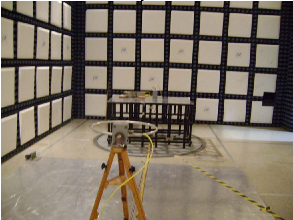
Test Set-up for Radiated Emissions – 6MHz to 30MHz – Horizontal Polarity
