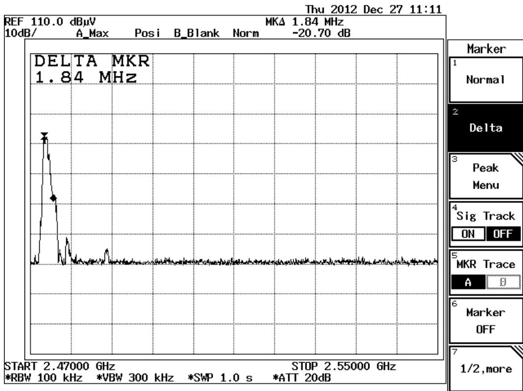
According to the page 13 of this report, the emission of the fundamental frequency 2472.83MHz is 82.9dB $\mu$ V/m and 56.7dB $\mu$ V/m for peak and average level respectively. Based on the delta method, the emission at the bandedge, 2483.5MHz, is more than 20dB below the fundamental. It is deemed to comply with section 15.215. Besides, it is below the limit of 74dB $\mu$ V/m and 54dB $\mu$ V/m for peak and average level under 15.209. It is deemed to comply with section 15.249(d).
