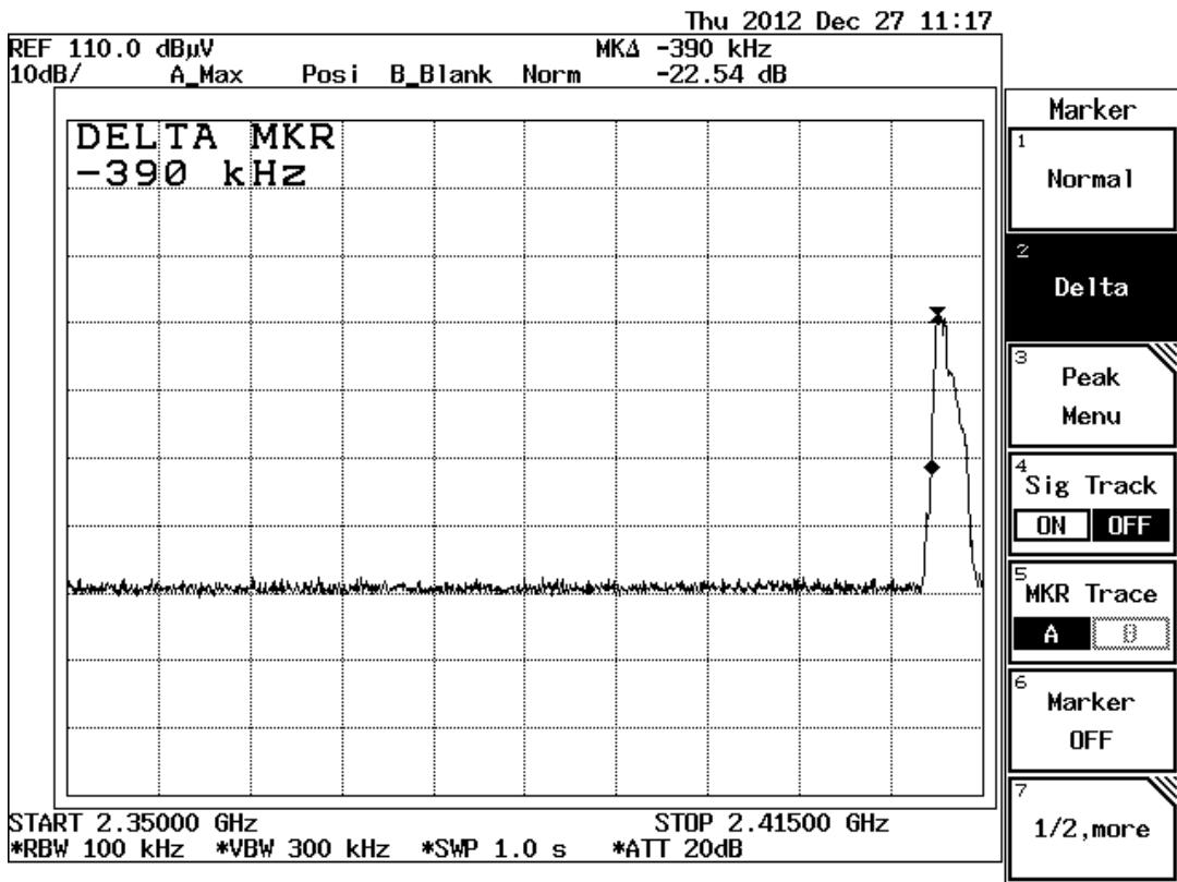
According to the page 13 of this report, the emission of the fundamental frequency 2411.92MHz is 82.1dB $\mu$ V/m and 56.6dB $\mu$ V/m for peak and average level respectively. Based on the delta method, the emission at the bandedge, 2400MHz, is more than 20dB below the fundamental. It is deemed to comply with section 15.215. Besides, it is below the limit of 74dB $\mu$ V/m and 54dB $\mu$ V/m for peak and average level under 15.209. It is deemed to comply with section 15.249(d).
